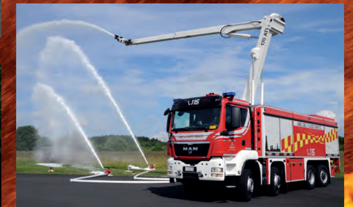
Large water tanker with compressed air foam system and extinguishing arm
