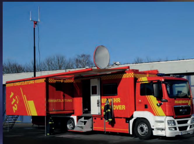
Mobile command unit MCU 3 acc. to German standard with side extension and satellite technology
